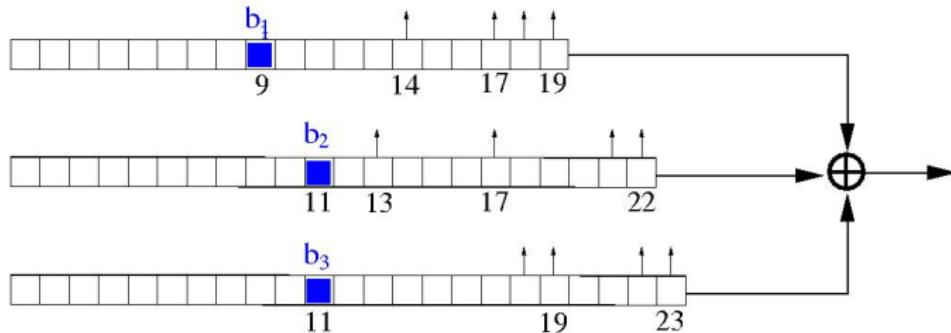
$$\text{posun}(i) = b_i \oplus \overline{T(b_1, b_2, b_3)}$$
